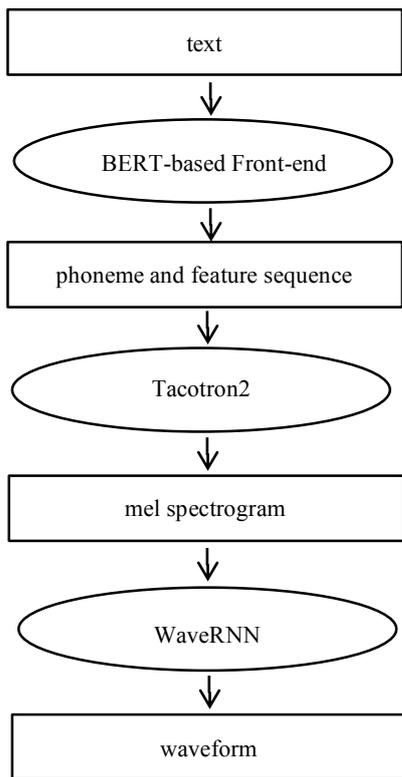
Figure 1: *The architecture of Ajmide TTS system.*
